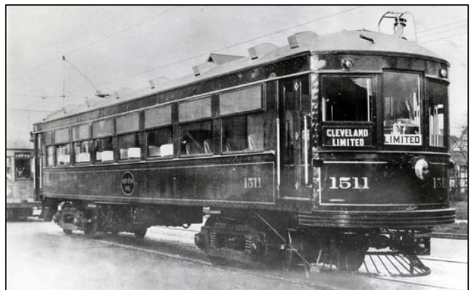
This type of coach, built by the Kuhlman Company, was used by N.O.T. & L. from 1921 until 1932. From the Summit County Historical Society Collection.
